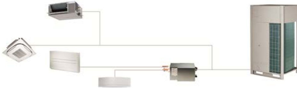
Figure 7-9: Example arrangement of multisplit equipment
