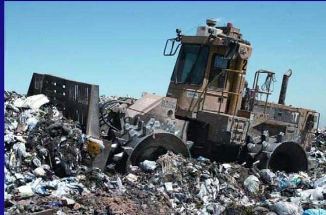
The instantaneous release due to landfill compaction can be estimated with 15 % of the CFC-11 content at disposal, which is equal to 11.4% of the total amount of CFC-11 in the appliances before shredding
